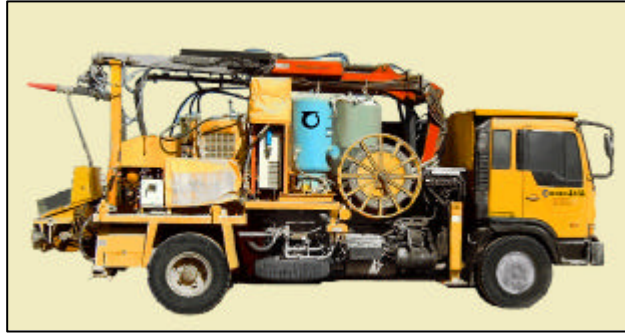
Fig.8 Shotcrete equipment using cement mineral type accelerator
